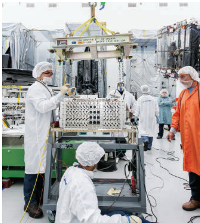
▲ Fig. 1 Digital payload of the Intelsat Epic NG satellite.
