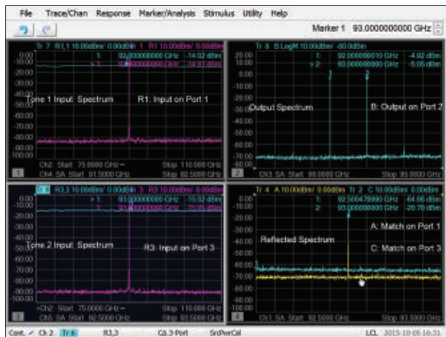
▲ Fig. 3 The single connection, multi-channel SA capability provides accurate, simultaneous measurements on all DUT ports.
